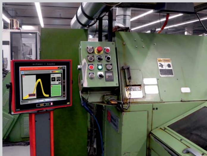
SK 800 load monitoring system with Foxmatic technology on a cold header at ITW
