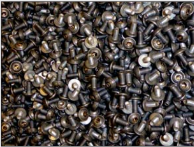
100 % crack free parts waiting for the thread rolling operation.
