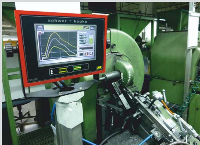
SK 400 load monitor in operation on a E. W. Menn planetary roller
