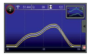
The Mandonic auto enveloping system adjusts the envelope limits perfectly according to the current variation of the process. The result: reliable detection of process errors with virtually no unnecessary machine stops.SKPuzzlemaster is provided for quick activatation of expert monitoring routines.
