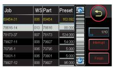
**Job Data**: start, interrupt, and finish jobs by simply selecting the desired job from the shown to-do-list on the terminal's screen. A virtual quick dial allows to page up and down the list speedily.
