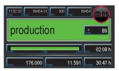
**Home screen**: shows current machine status and production rate, current job progress, and remaining run time to finish the job.
