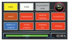
**Down codes**: select the desired down code from your individually assigned list of possible reasons. If desired, you can even lock the machine in case no down code is entered.
