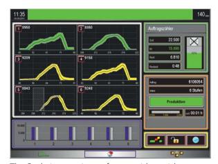
The Cockpit operating surface provides quick access to all important functions. Horizontal and vertical navigation features and short cut buttons make the use of the monitor extremely simple. User access can be controlled by RFID key to avoid unauthorized alterations of parameters and settings.
